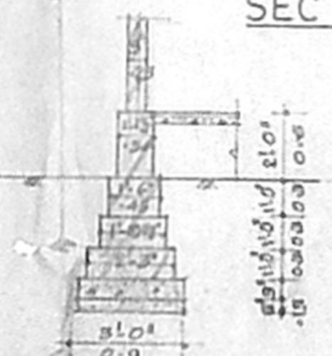
FOUNDATION DETAIL AT (A)
